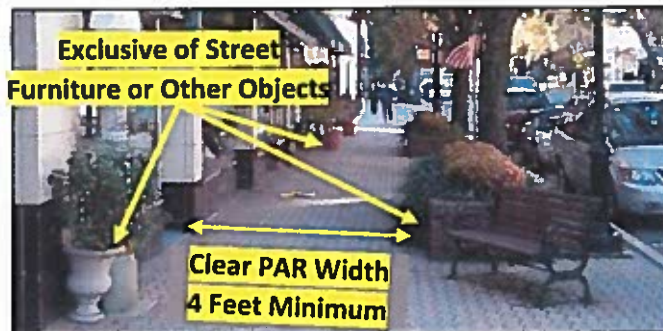
Figure 5: PAR Width and Street Furniture
