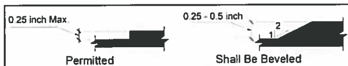
Figure 17: Vertical Surface Discontinuity
