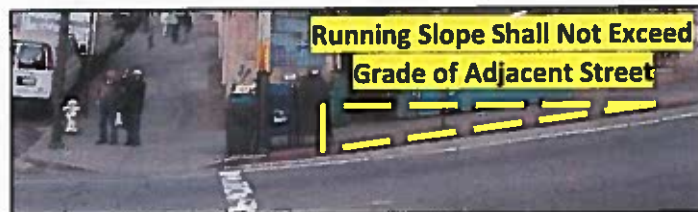
Figure 9: PAR Running Slope Shall Not Exceed Grade of Adjacent Street
