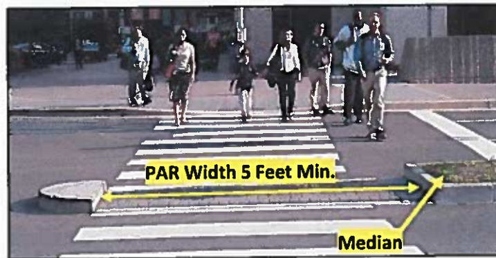
Figure 70: PAR Width within Pedestrian Street Crossings
