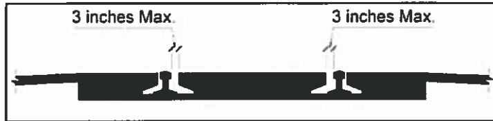
Figure 20: Flangeway Gaps on Freight Rail Track
