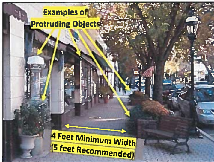
Figure 21: PAR Clear Width Excluding Protruding Objects
