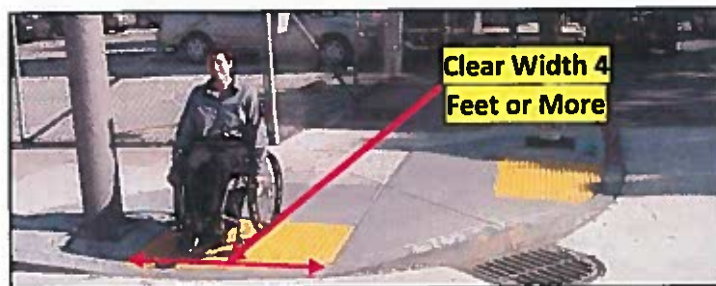
Figure 32: Curb Ramp Width
