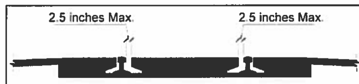
Figure 19: Flangeway Gaps on Non-Freight Rail Track
