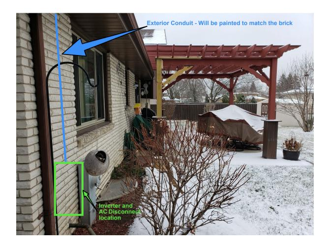
The DC wire on the roof will be run through the attic. Depending on the structure of the attic, the rest of the DC wire run will come out either the wall or the soffit above the meter. This conduit will be painted to match the color of the brick as much as possible. This is all located in the back of the residence and will not be an eyesore.
